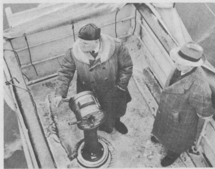
From the bridge of the "N.B. McLean", Captain Charles Caron, master of the vessel, telegraphs his needs to the engine room, as he tackles the job of clearing a path through the ice on Lake St. Peter. Herbert Land of the St. Lawrence Ship Channel looks on as the "N.B. McLean" charges and lunges through ice formations along the Ship Channel. Any day now, the "N.B. McLean" will arrive at the Port of Montreal after having loosed King Winter's icy grip from this all important strip of Canada's main highway of water-borne commerce.
