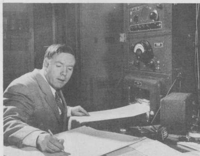
Intricate radio recording instrument takes down radio signals sent by radiosonde technician on three different frequency pitches, each in turn recording the humidity, temperature and barometric pressure. H. J. McCabe records and codes the information.
