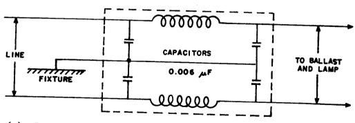
(v) In many cases a split capacitor of  $0.1\,\mu\text{F}$  capacitance for each section may be connected at the entrance to the fixture, with the centre point connected to the fixture and the other two leads to the lines. This may be found to give adequate suppression.
