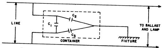
For BX cable, all capacitors are approximately 0.07  $\mu\,F$  ; for open wiring C  $_1$  is 0.02  $\mu\,F$  and C  $_2$  and C  $_3$  are 0.002  $\mu\,F$  .
